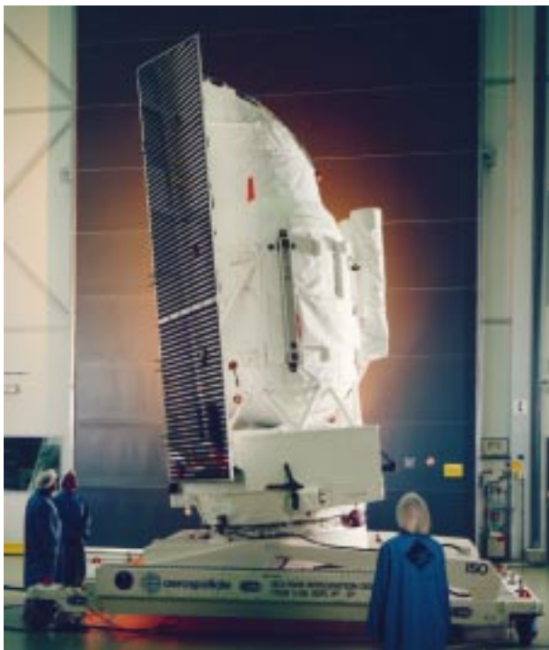
Fig. II.14: The 5.4-metre long Infrared Space Observatory, ISO, in the assembly hall at Aerospatiale. 2300 litres of superfluid helium cool the entire satellite down to near absolute zero. (Photo: DASA)
