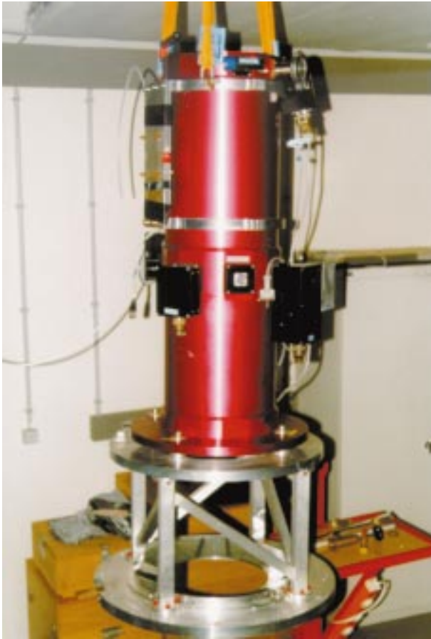
Fig. III.6: OMEGA Prime's CCD unit.
