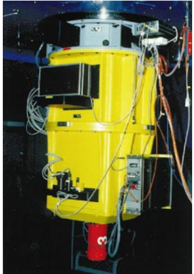
FIG. III.3: The MOSCA infrared camera in operation.
