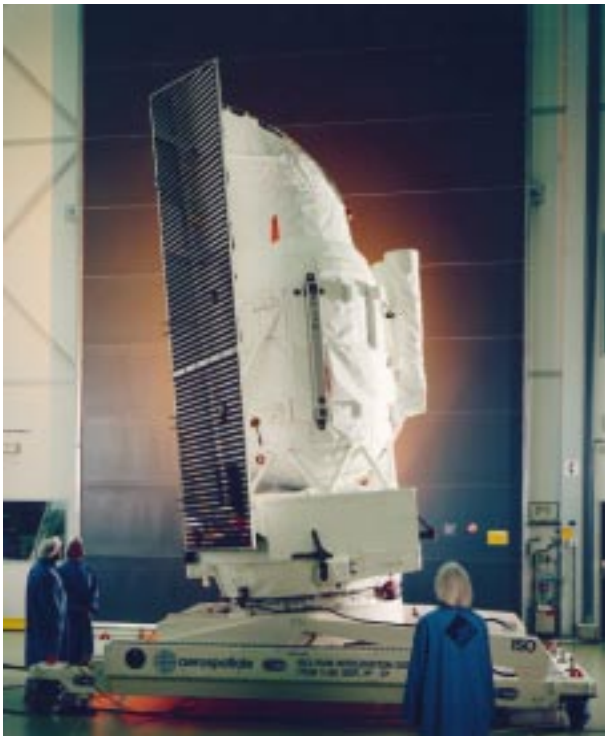
Fig. I.3: The ISO satellite was 5.4 metres tall and weighed 2.4 tonnes. The telescope and the aperture system were cooled down to 1.8 Kelvin with helium gas, which evaporated from a tank containing 2300 litres of superfluid helium.
